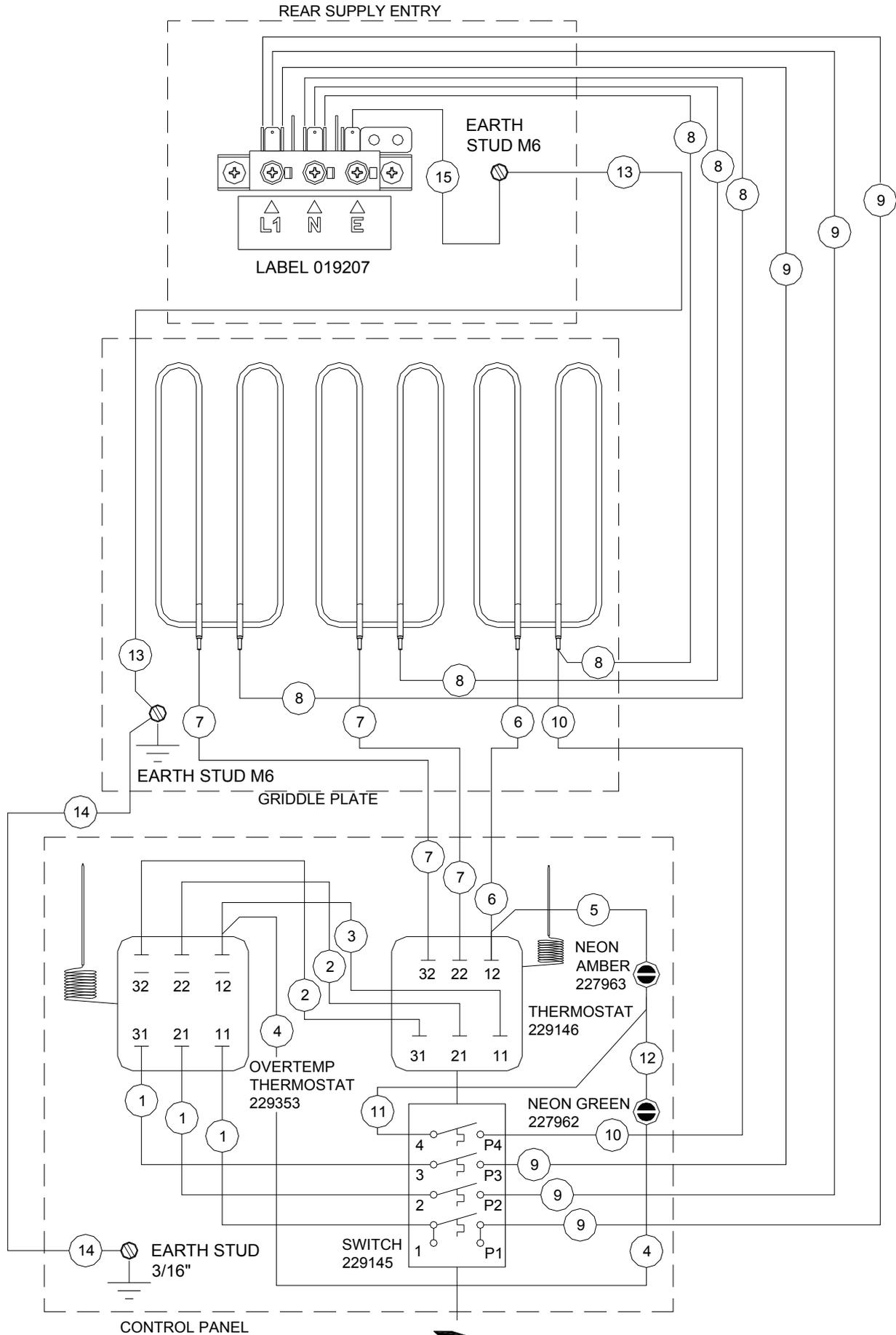
EP516 Wiring Schematic
